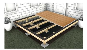
Z Start by laying out your Decking Boards onto the desired area before fixing them in place. Ensure there is a 3mm gap between any Boards at butt ends or side by side and between all walls and fences.
