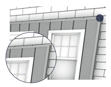
Once the Corner Trim is cut to size, you can use CT1 Adhesive along one or both sides of the Corner Trim to attach it to the edge of the Cladding.
